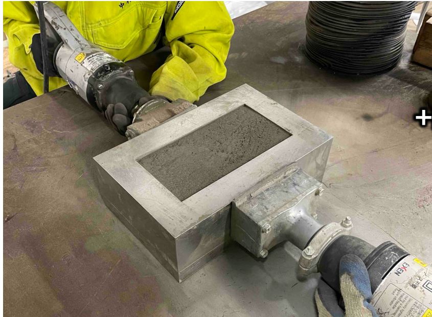
Vibration applied before pressing
