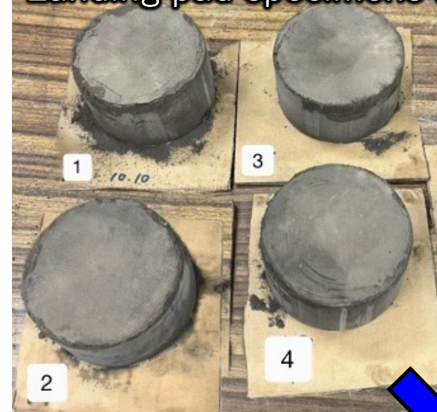
Landing pad specimens before compressive test
