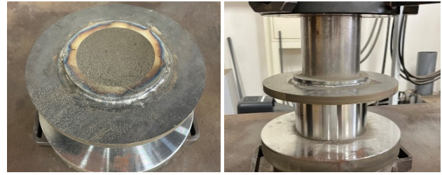
Fig.2. Regolith Placed in the Mold and the Compaction Process
